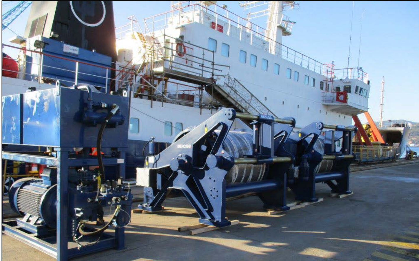
Winch and HPU supply (Ibercisa)
